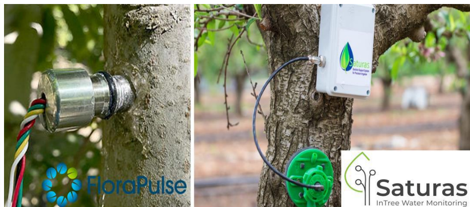
Figure 2: FloraPulse (left) and Saturas (right) sensors for measuring stem water potential embedded into tree trunks
